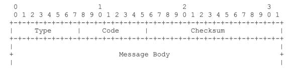
The type field indicates the type of the message. Its value determines the format of the remaining data.
